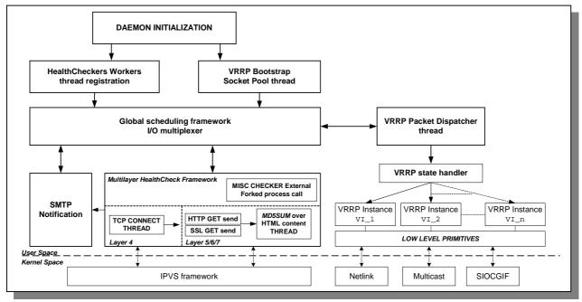
The following figure illustrates the Keepalived internal software implementation components. Keepalived uses a fully multithreaded framework based on a central I/O multiplexer. The 2 main components are:
