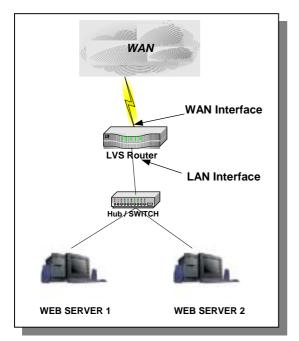
LVS stands for "Linux Virtual Server". LVS is a patched Linux kernel that adds a load balancing facility. For more information on LVS, please refer to the project homepage: <u>http://www.linux-vs.org</u>. LVS acts as a network bridge (using NAT) to load balance TCP/UDP stream. The LVS router components are:
